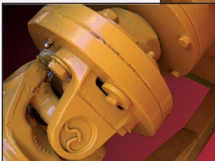
Two sets of shear bolts protect the impeller and the augers.
